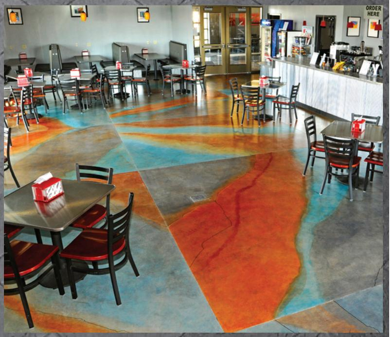
Brickform's® suite of decorative stains provide permanent, long lasting color to concrete surfaces. Both the ARTesian™ water-based stain and E-Stain™ reactive stain, prevent exposure to Volatile Organic Compounds or VOCs.
